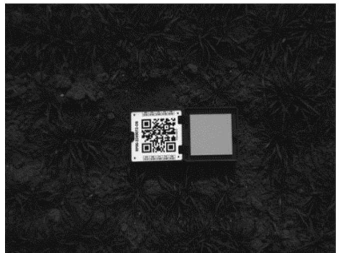
**Figure 3** Calibration plaque with known reflectance. This image is captured before each flight and is instrumental in obtaining physically accurate spectral measurements.
